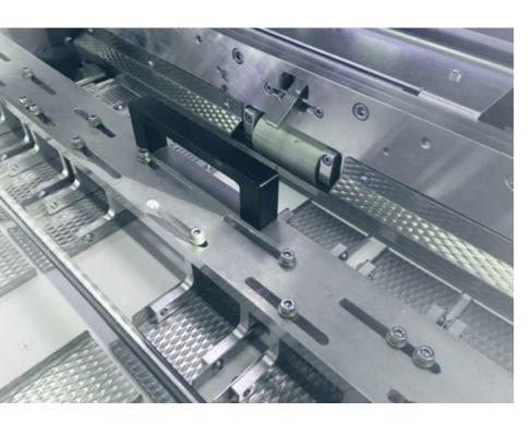
Highly stable paper path, running up to 60,000 documents in A4 per hour. Multi gains up to 4-up can be processed at a web width of 560 mm. Gross formats will be cropped 4-sided to the net format. The cutter works at the horizontal (slit and gutter cut) and vertical cuts at full speed. Waste sheets will divert by the whitepaper-management. The use of highly durable knives allows long maintenance intervals.
