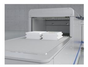
The grouped documents are accelerated and placed on the stacker separated into groups. The stacks can be deposited on the delivery belt without getting caught up in one another. It is therefore easy for the operator to remove the stacks. When the end of the stack is reached, the stacks are passed onto the next delivery belt. Through an integrated clipboard the system works also while stack exchange without interruption. The height of the stack is around 2,000 sheets at 80 g/m².
