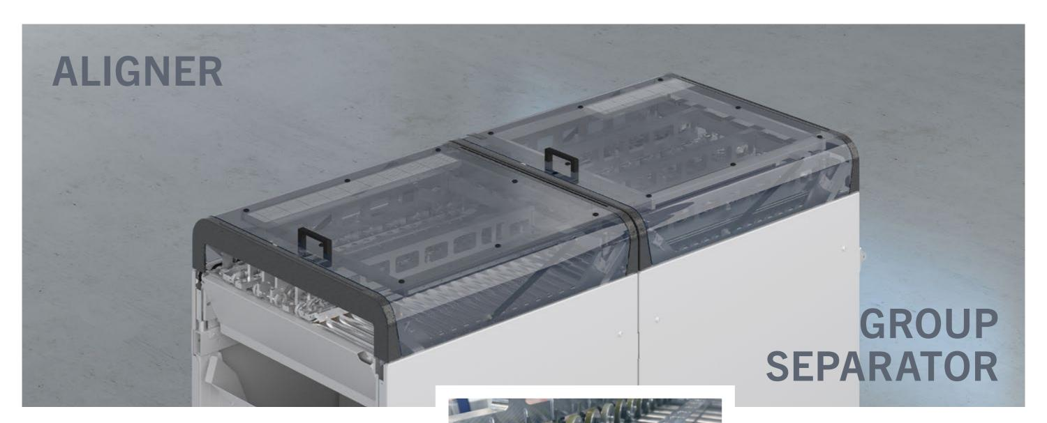
The cut to final format documents are isolated horizontally and aligned vertically. Thus, 2-up to 4-up applications can be processed without longitudinal cut-outs. The productivity can be increased by over 30 percent especially with books or the American Invoice 5 ½ format, that are not printed full bleed.
